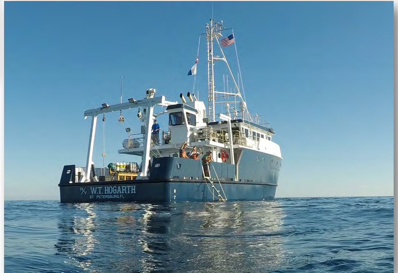
R/V W.T. Hogarth 78 feet, capable of multibeam and video missions
